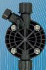
Polypropylene pump head complete with ball valves (ceramic balls) FPM or EPDM seals
