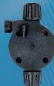
PVC pump head for high flow rate ( 20 lt/h up to 50 lt/h) complete with ball valves (ceramic balls) FPM or EPDM seals
